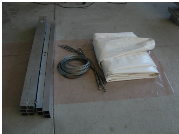
Fig. 2 Compression element, cables and inflatable hull of a single girder of the Tensairity demonstration bridge with 8 m span
